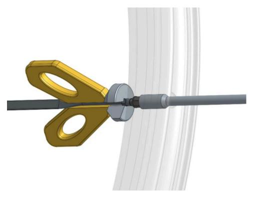
When centering, the spoke must be countered from the inside with a centering wrench.
